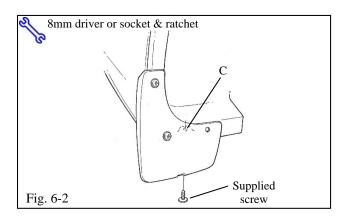
(b) Hold the mudguard up and into the bumper panel and install a supplied screw in location C, then tighten (Fig. 6-2). Do not overtighten the screw.
