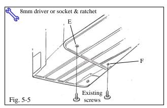
(g) Reassemble the bumper panel and liner then reinstall the preexisting screws in locations E and F (Fig. 5-5).
