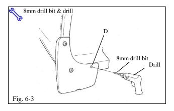
(c) Hold the mudguard tight to the liner and use the part as a template to drill an 8mm hole in location D (Fig. 6-3).
